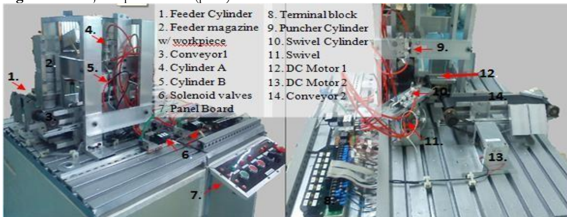
Figure 3A: Project Specification (parts)
